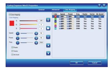
Color mapping is used to define multiple settings within 1 design file. The speed, power and frequency work in the same as in the general options.
