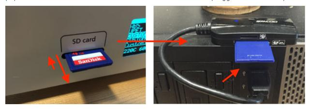
You can then click on the floppy disk icon in the upper left hand corner to save the gcode to the SD card. If there are other memory devices in use (like flash drives), Cura will ask you which device to save the file to. You can find out which letter drive is the SD card by opening a Windows File Explorer window and looking at the files present on the drive. (It's usually the G drive).
