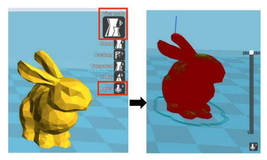
Once in the layer-viewing mode, you can drag the slider up and down to view different layers of the model. It will show you the current layer and everything below it. Clicking the small icon below the slider will switch it to single layer mode. Red is the outer perimeter of the part, green is the inner perimeter, yellow is infill, and teal is support.
