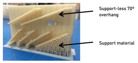
The UM2 has a single nozzle and a single material. Therefore, the system uses Same Material Support Material (SMSM), otherwise known as Breakaway Support Material (BSM). The machine perforates the interface between the support and model, making the support easy to tear off afterwards.
