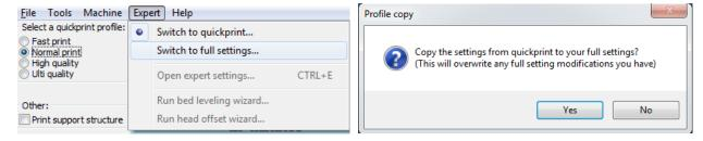
Once you are in the Full Settings mode, you can load the default settings profile by going to *File, Open Profile...* You should navigate to the Desktop and select the **UM2\_DEFAULT\_PROFILE.ini**.
