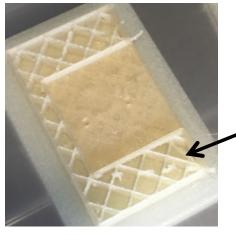
Part interior cavity is filled with a lattice structure of specified density
